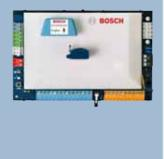
The control panel has an integrated telephone digital communicator. It provides local and remote dual tone multifrequency (DTMF) control, a digital communicator (SIA, Contact ID, Voice, Fast Format) and personal messaging formats (Voice and SMS Text Messaging). Terminal strips are color-coded and each input and output has a dedicated pair of terminals. The programming key and ROM update key support a "hot" plug-in and perform actions automatically.
